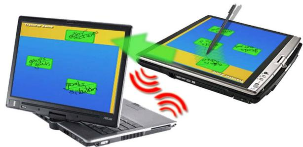
Figure 6. Two Tablet-PCs activate an “exchange zone” when they approach each other
